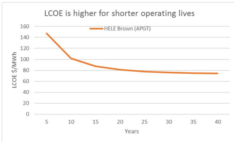
Figure 5 - Levelised costs for a brown coal generator, recalculated for operating lives between 5 and 40 years
